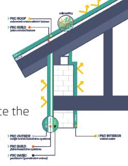
The thermal resistance and insulating and reflective properties create a synergistic effect in reducing surface heat transfer. The coating has excellent insulating properties.
